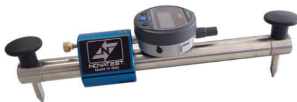
Figura 2-3 deformometro DN250-10 NOVATEST
